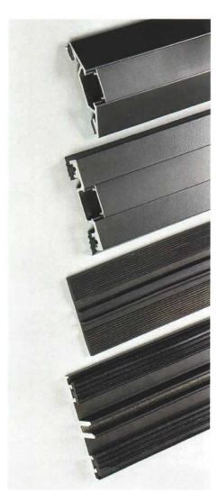
Pros and cons. Baseplates can be aluminum or EPDM rubber. Aluminum provides a stable bearing surface for glazing but can be time-consuming to install, and it is subject to interior frosting. The EPDM doesn't frost up but doesn't have a condensation gutter. Photo by Susan Kahn.
